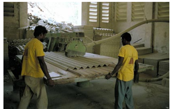
Workers at AA mines in Zimbabwe cutting sheets containing Zim asbestos
